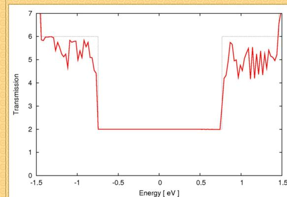
Calculated transmission probability against the energy for (6,4)@(10-10) double-walled carbon nanotube (*Fermi energy is shifted to 0*).
