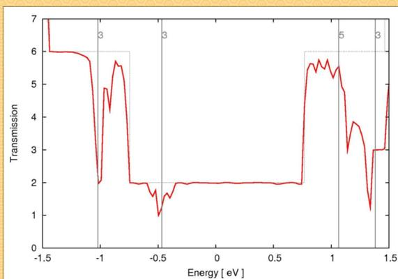
Calculated transmission probability against the energy for C<sub>60</sub> filled (10-10) carbon nanotube (*Fermi energy is shifted to 0*).
