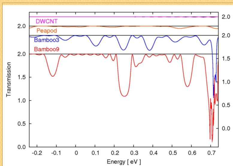
High resolution calculation of transmission probability vs energy for comparison of key transport signatures. (Note that the curves are shifted vertically for better visibility).
