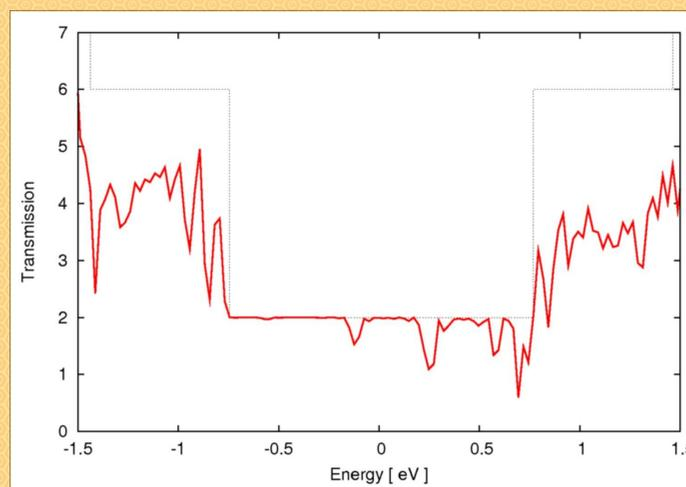
Calculated transmission probability against the energy for a 293.93 Å long (6,4) left-right nanobamboo with 9 bumps in (10-10) nanotube (*Fermi energy is shifted to 0*).
